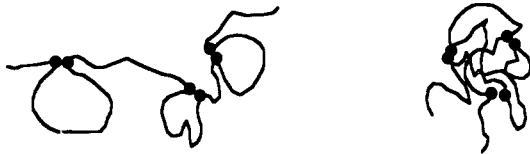
Figure 3. Local versus global sticking. The left-hand sketch shows the extreme of local sticking: only chemically adjacent stickers are associated. In the right-hand sketch stickers are associated independent of their position along the chain.
